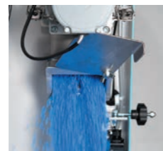
残材抜き Extraction of Remaining Materials
